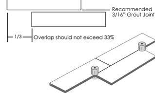
Use a leveling system during installation to reduce lippage
