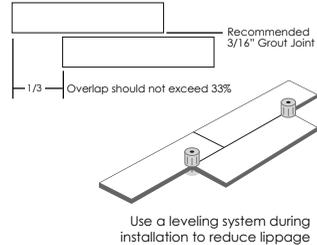
Use a leveling system during installation to reduce lippage
